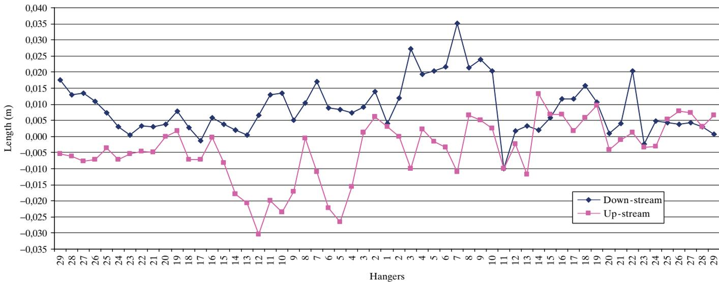
Fig. 14: Hanger's length difference between design and measured value after second tensioning
