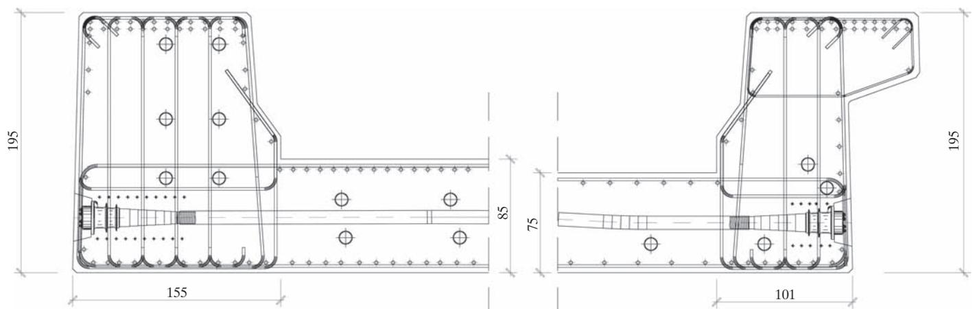
Fig. 3: Detail of cross section (slab and edge beam) near the obtuse (left) and acute angles (right)
