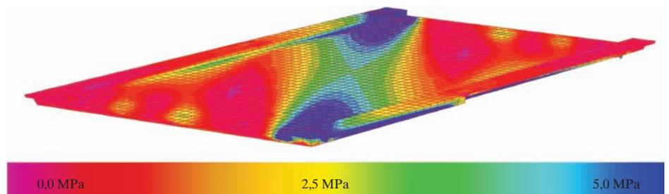
Fig. 2: The slab mesh and the principal tensile stress under service loads
