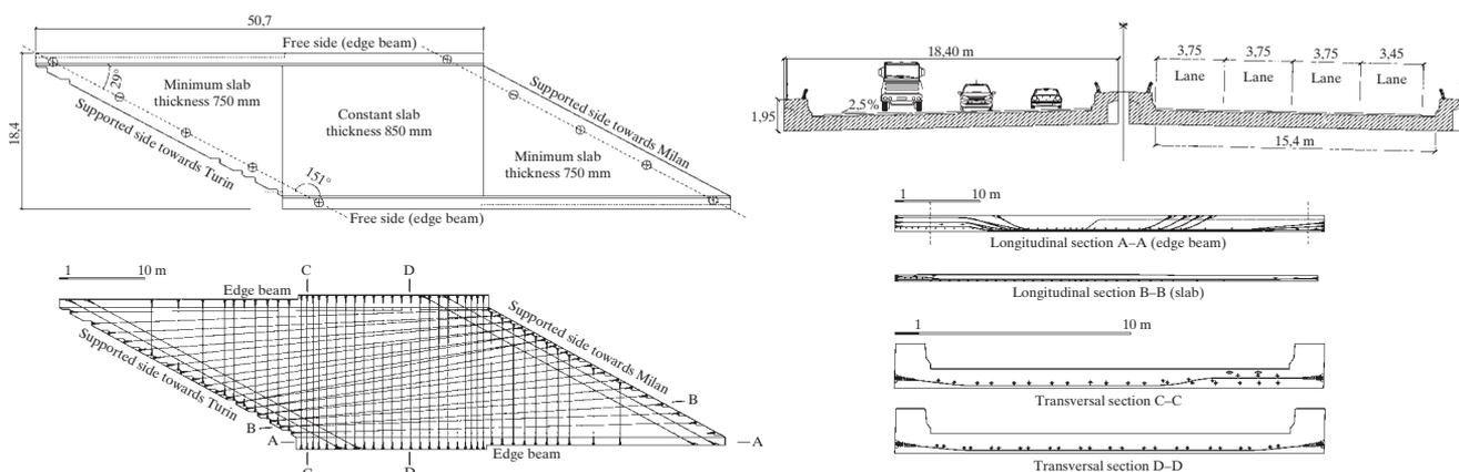
Fig. 1: Slab geometry and prestressing layout
