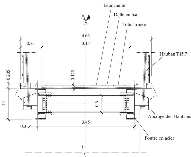
Fig. 5: Cross section of new composite deck (Units: [m])
