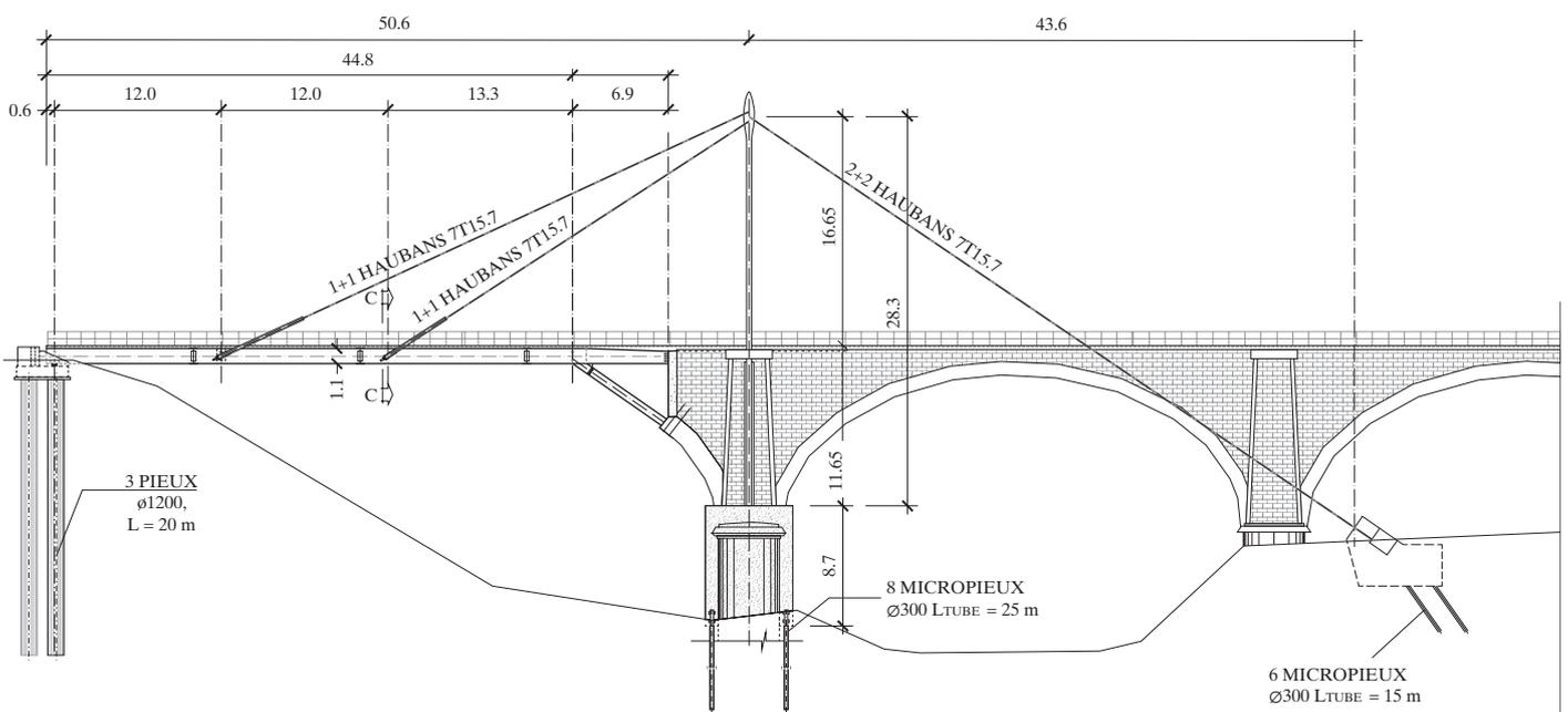
Fig. 2: The longitudinal profile of the new Student Bridge (unit : m)
