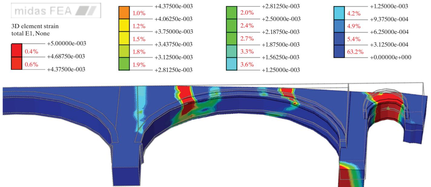
Fig. 4: Total positive (traction) strains, with finite elements percentage, caused by the imposed foundation slippage (Units: [-])
