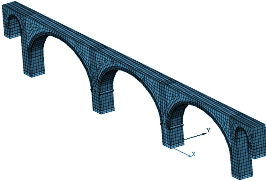
Fig. 3: The finite element model of the Student Bridge before the collapse
