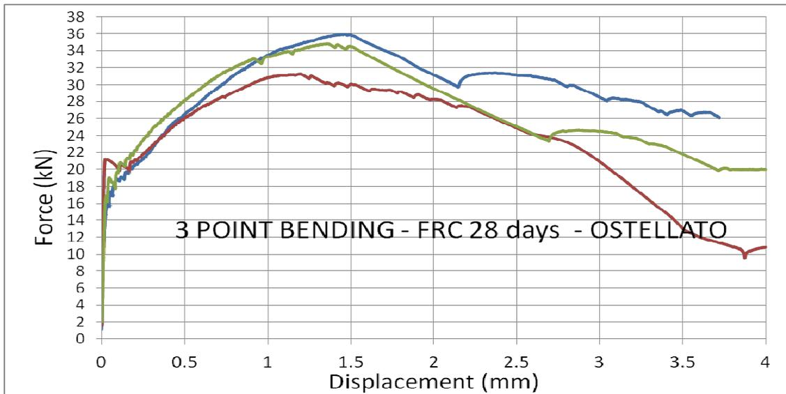
*Fig. 4: Test result of FRC notched beams*
