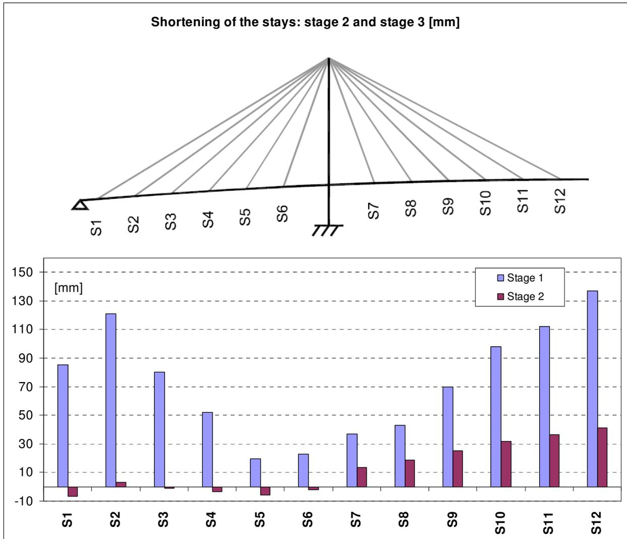
Fig. 6: Shortening (mm) of the stays for stage 2 and 3 (half bridge).
