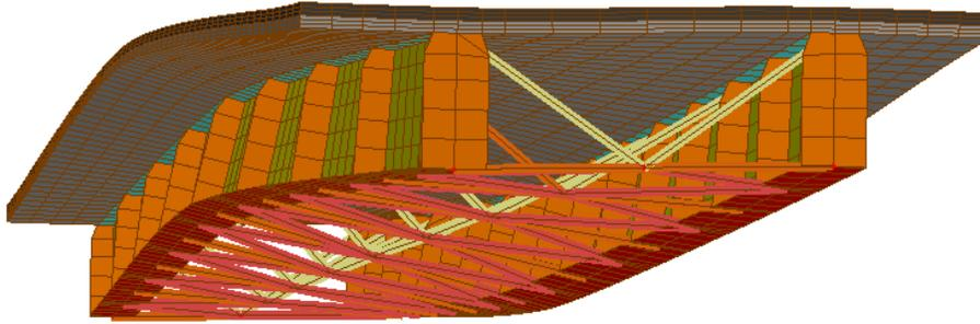
Figure 6: Deformed shapes for the single span case. Torsionless and horiz. braced
