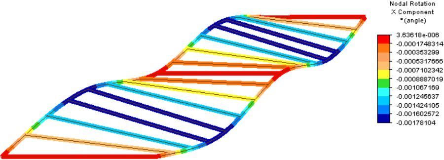
Figure 8: Grillage analysis of the 2 span case.
